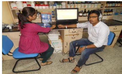
Figure 2: Biopac Systems for Biomedical data (EOG, EMG, heart rate variability, stress test, reaction test, etc.) acquisition and analysis.
